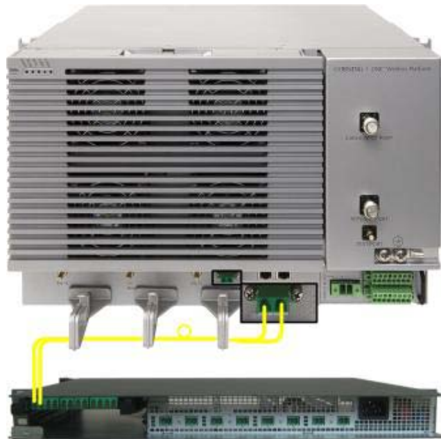
Figure 4-15 Fiber Connections Towards ICU
