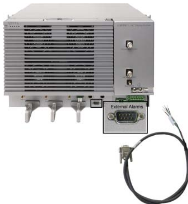
Figure 4-17. MRU External Alarms Connector and Cable
