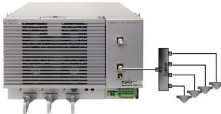
Figure 4-16 Example of MRU Connections to Broadband Antennas (Via Splitter)
