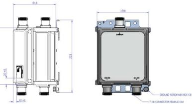
Dimensions - Single Unit with Auto-Sense and 7/16-DIN Connectors
