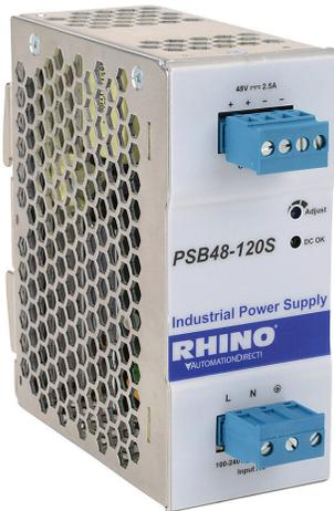
RHINO SELECT PSB series switching power supply, 48 VDC @ 2.5A/120W (adjustable), 120/240 VAC or 120-375 VDC nominal input, 1-phase, enclosed, aluminum housing, 35mm DIN rail mount, removable screw terminal, hazardous location rated.
