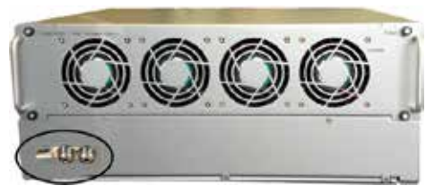
Figure 6. Grounding Lug (Chassis Rear)
