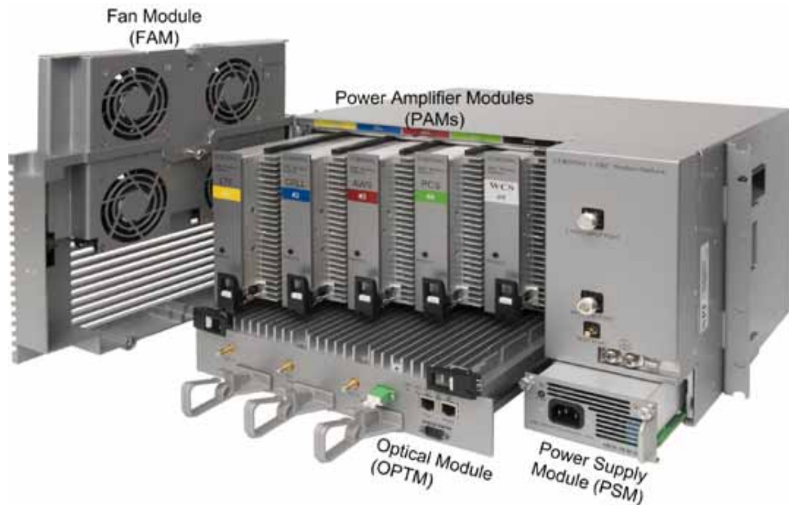
Figure 2-13 MRU Main Modules
