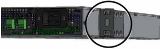
Figure 5-3. PSU6 Rack Bracket(s) for Removal
