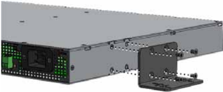
Figure 5-4. DC Assembling Wall Mount Brackets
