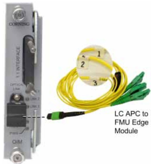
Figure 4-21. OIM Fiber Connections
