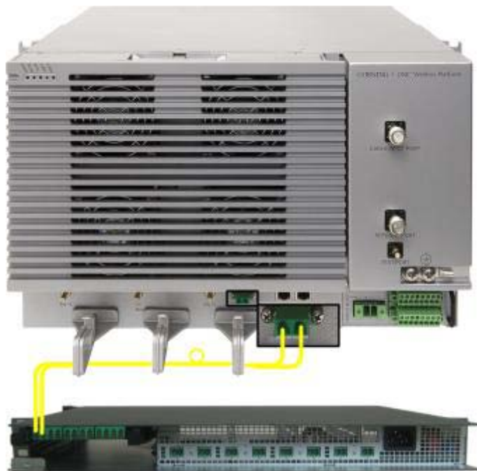
Figure 4-6 Fiber Connections toward ICU
