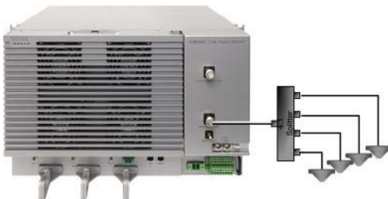
Figure 4-7 Example of MRU Connections to Broadband Antennas (Via Splitter)
