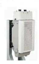
A distributed eNodeB expands deployment options by using two components, a Base Band Unit (BBU) containing the digital assets and a separate RRH containing the radiofrequency (RF) elements. This modular design optimizes available space and allows the main components of an eNodeB to be installed separately, within the same site or several kilometres apart.
