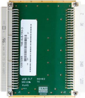
Extender Board (TME-SUB-TRX-D)
