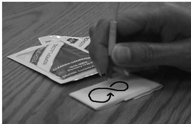
Figure A-1 Cleaning the ferrule endface
