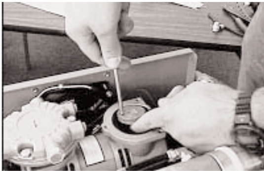
Remove the two screws securing the piston retainer plate and cup. Discard the old cup, retainer, screws and both gaskets.
