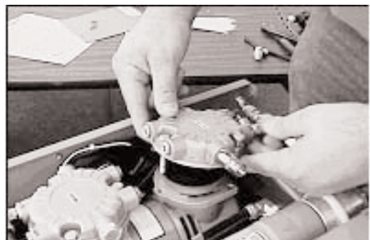
Replace the valve plate and pressure head. Tighten bolts.
