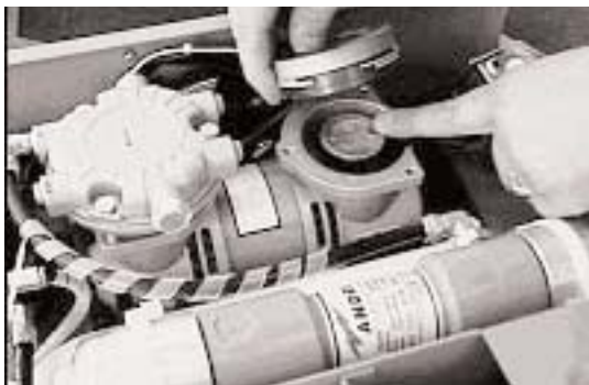
Add all shims included in the kit (some kits may not have shims) to the original stack and replace the piston sleeve.
