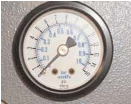
Pressure Gauge - indicates dehydrator output pressure in psi and kPa.
