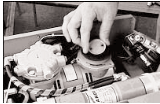
Install the new piston cup by aligning the holes with those in the piston and pushing it into the piston sleeve.
