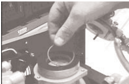
Install new gasket between cylinder and valve plate.
