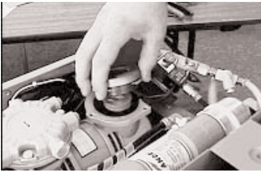
Remove piston sleeve. Be careful not to damage any of the shims when removing the piston sleeve.
