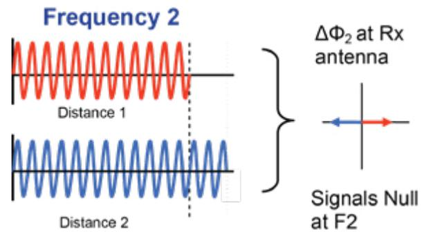
Figure 9: Two path sample at frequency 2.
