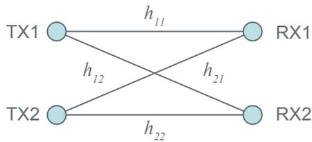
Figure 11: 2x2 Multiple antenna configuration.
