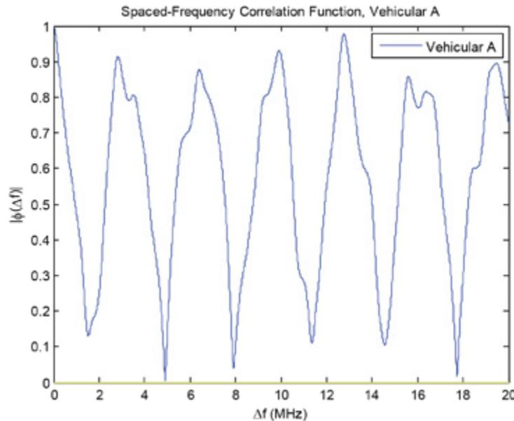
Figure 16: Spaced-frequency correlation function.
