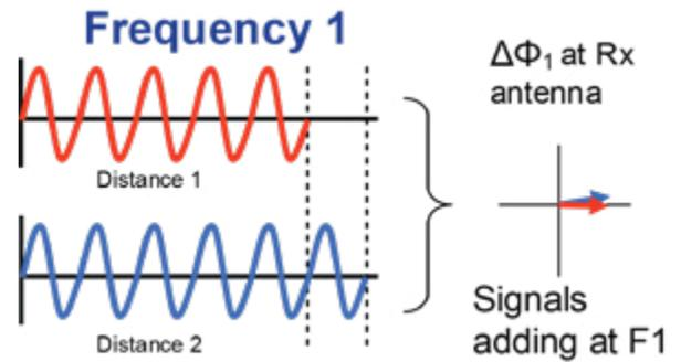
Figure 8: Two path sample at frequency 1.
